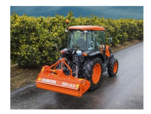
More power and performance for all tasks is the motto for the lift linkage of the M5001N. Thanks to its stable category II 3 point hitch, the tractor can lift heavy equipment with ease. 2,300 kg lifting capacity speak for themselves. You will really appreciate the additional lifting capacity in areas where your previous tractor reached its limits.
