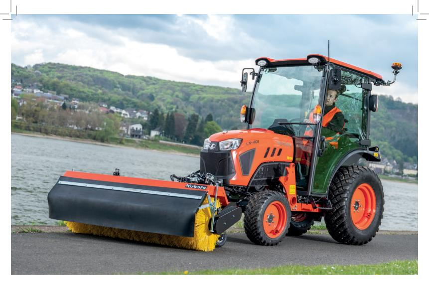
Quieter and more economical at the touch of a pedal Thanks to the tractor's auto-throttle function, you can synchronise driving speed and engine speed with just one pedal. This simplifies operation, reduces noise emissions and keeps fuel consumption low.
